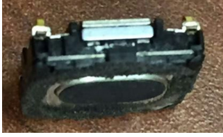
Fig. 5. Audio transducer that sits below the ear-mesh.
